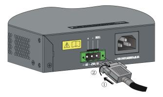
Step4 Connect the other end of the RPS DC power cord to the external RPS power supply system.
